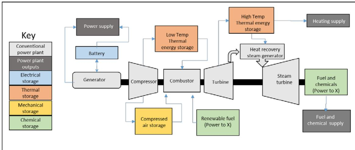
The chart below shows example storage solutions that can be combined with thermal power plants in the short-, medium- and long-term. Solutions are shown in the thermal, mechanical, electrical and chemical areas. For example:
