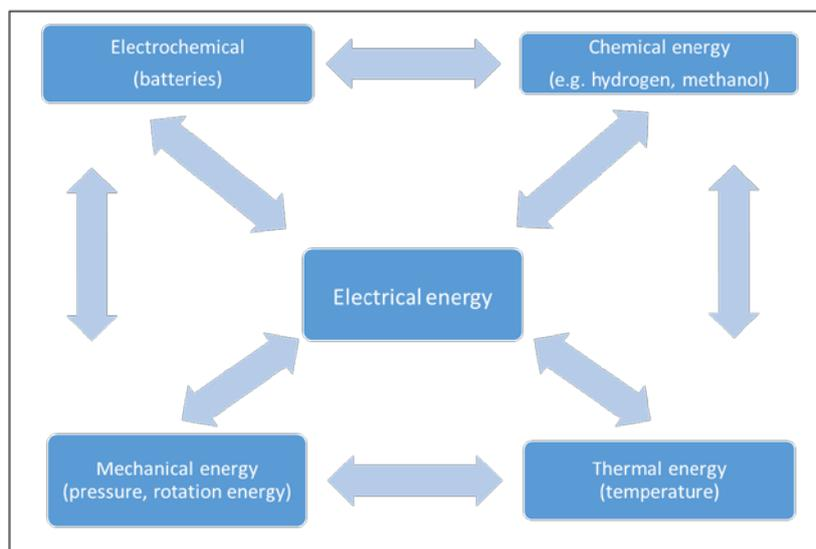
Energy storage can be simplified into four dominant forms that are interchangeable between each other: electrical, thermal, mechanical and chemical storage. The cost and efficiency to transform between the energy forms is determined by the available technology. The size and duration of the storage also has a large impact on the cost and performance. These factors combine to determine if storage options are available and economically viable to meet power management requirements.
